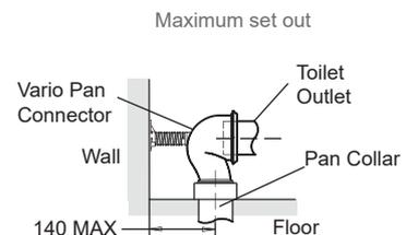
\*Note: Set outs between 160-240 mm are achievable with the Long Adjustable Vario Connector 77837A-NA (not supplied).
