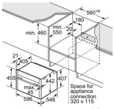
measurements in mm
