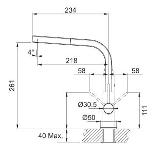
**PLEASE NOTE:** Large and heavy taps should ideally be mounted directly through the solid benchtop or fully supported from underneath. For all other swivel taps, we recommend the use of the Franke Tap Support Arm to provide additional support. Please ensure all Franke tapware is installed at a pressure of no greater than 500 kPa in accordance with AS/NZS3500 and insist that your plumber flushes all of the water supply lines before installing tapware. Failure to do so may void warranty.
