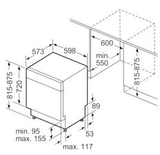
measurements in mm
