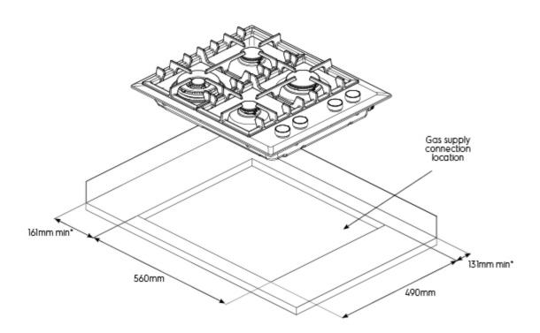
${}^*\text{To}$  combustible surface (dimension is not relevant if the adjacent surface is non-combustible).
