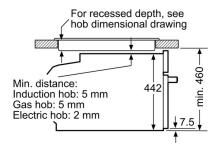
measurements in mm
