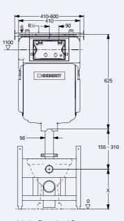
$In-wall\ cistern\ installation\ diagram\ shown.\ For\ in-ceiling\ and\ in-duct\ installation\ diagram\ s,\ please\ visit\ the\ Download\ Centre\ at\ geberit.com. au\ and\ search\ 'remote\ button\ installation'\ or\ call\ 1800\ GEBERIT.$
