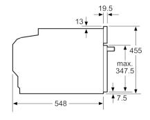
measurements in mm
