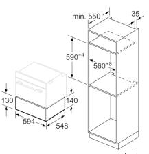
measurements in mm
