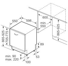
measurements in mm
