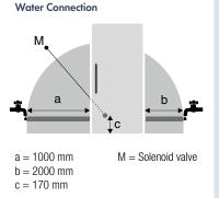
Plumbing must be installed adjacent to the side of the appliance which contains the IceMaker.
