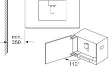
If using the 92° hinge limiter (spare part no. 00636455), the minimum distance to the wall is only 100 mm. measurements in mm
