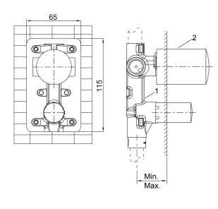
Flush the water supply pipes thoroughly to remove debris before installation. Shut off the main water supply. Determine a suitable location on the wall to install the valve body.
