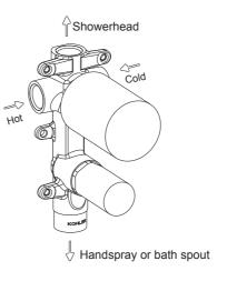
Supply enough tape or sealant to all connections. Connect R1/2" hot and cold supplies, showerhead and bath pipings to valve body. Connect hot supply to the end on the left.
