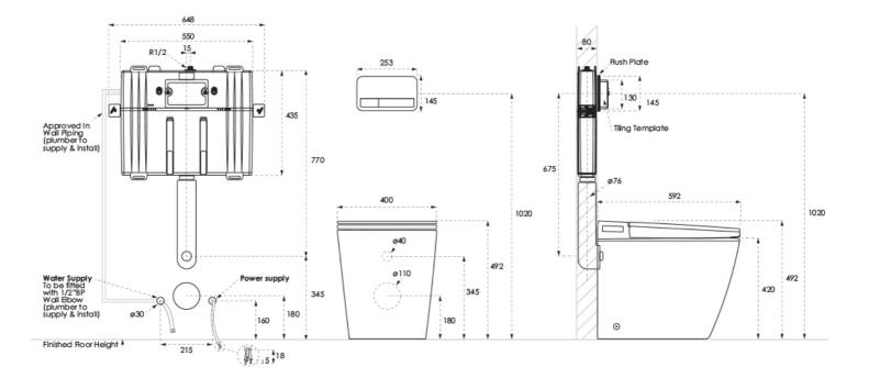
Note: All dimensions are in millimetres and are subject to normal manufacturing variations. Always use the physical product measurements for cut-outs and rough-ins as the technical details shown may differ from the actual product. Use acetic cured silicone sealant. Do not use epoxy type adhesives. Clean with damp cloth. Do not use abrasive cleaners, liquids or pastes.
